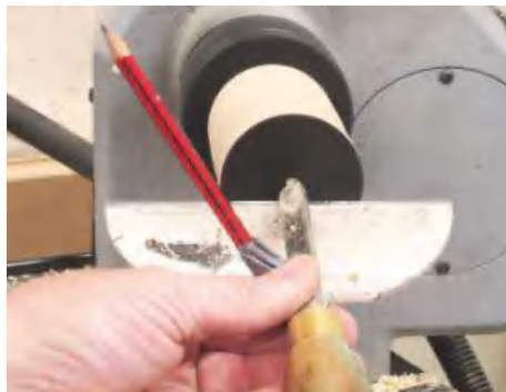
▲ Pic.13 Hollowing egg cups, boxes, etc. is best done with the spindle gouge. The pencil shows the 11 o'clock position of the flute of the tool
